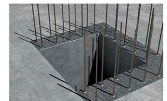
Post-installed rebar connections
