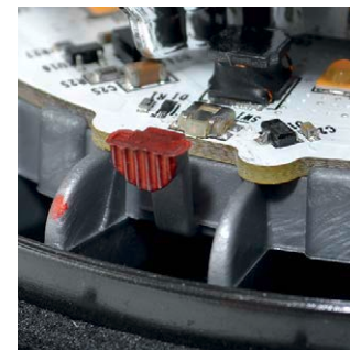
Internal red switch to be operated manually
